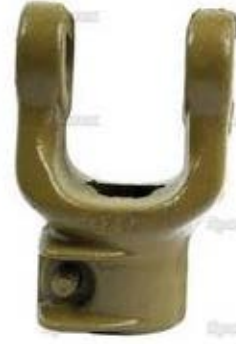
品名 PTO Yoke - Quick Release (U/J Size: 30.2 x 79.4mm) Spline Type: 1 3/8"x 6 品番 SPX S.6118
