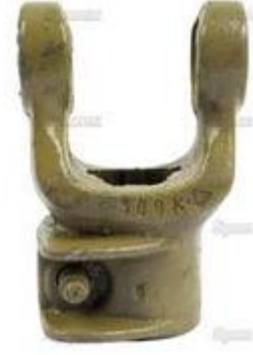
品名 PTO Yoke - Quick Release (U/J Size: 27 x 70mm) Spline Type: 1 3/8" x 6 品番 SPX S.6018
