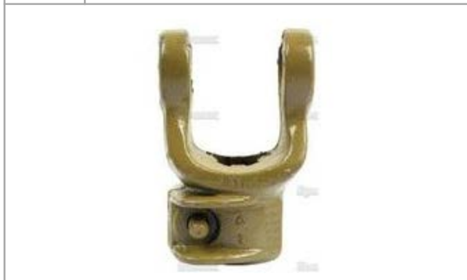
品名 PTO Yoke - Quick Release (U/J Size: 27 x 74.5mm) Spline Type: 1 3/8"x 6 品番 SPX S.6048
