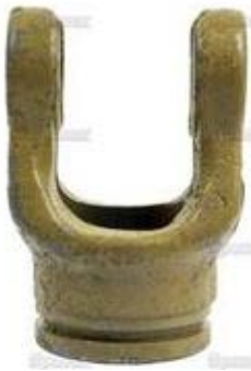
品名 PTO Yoke - Tube Yoke (U/J Size: 30.2 x 79.4mm), Profile: Triangle, Size: 51.6 x 3mm, Ref: 12510. 品番 SPX S.6111
